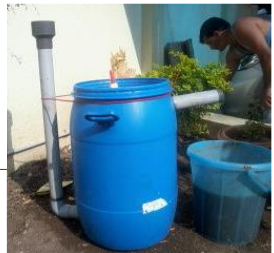
Figure 27: Home made biogas plant 250L, source: http://www.instructables.com/id/Biogas-at-home-Cheap-and-Easy/
